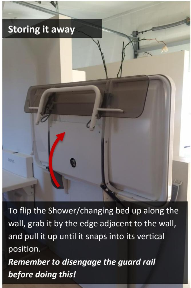
To flip the Shower/changing bed up along the wall, grab it by the edge adjacent to the wall, and pull it up until it snaps into its vertical position.
