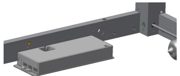
6.1.6 Attach control unit to angle plate and fasten.
