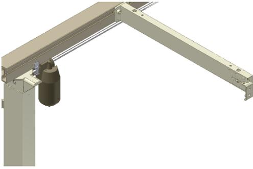
7.1.5 All support arms, but 2, may be pushed into the aluminium profile from the right hand side to the required position and fastened with two screws on each support. We recommend a maximum distance between the support arms of 60 cm / 23.6in in order to obtain optimum stability.
