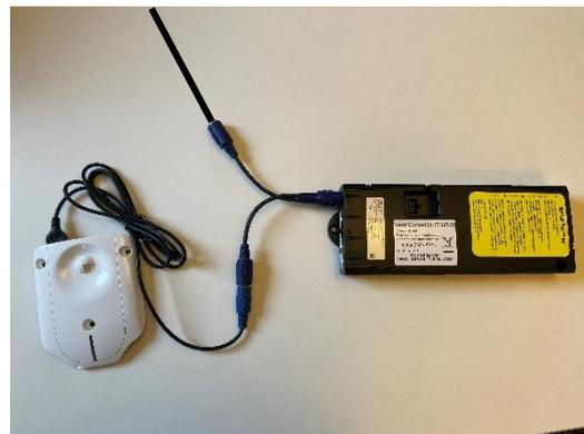
8.7.2 Insert the split-cable in the plug "HS" in the control box. Then, insert the adapter in one end of the split cable, and the button that came with the product, in the other
