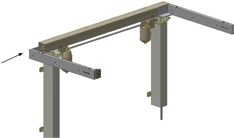
8.6.1 Push support arm into aluminum profile and make sure support arm is level with profile. Afterwards tighten screws. By using this support arm it is possible to mount hotplate or sink closer to edge of tabletop.
