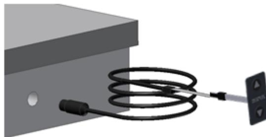
7.9.1 The control switch for the height adjustment must be fitted in the wooden front fascia. It consists of a control switch with a 1.5 m / 59 in long cable provided with a DIN plug for the control switch. Choose the required position in the front fascia and drill an 18 mm / 0.7 in dia. hole in the fascia. Push the cable through the hole in the front fascia from the front.
