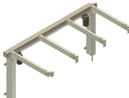
7.1.10 The right hand side support arm may be pushed into the profile, positioned direct on top of the left leg, and fasten it.
