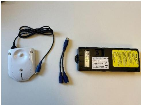
8.7.1 Determine the placement of the adapter, then grab the Bluetooth adapter and the split-cable
