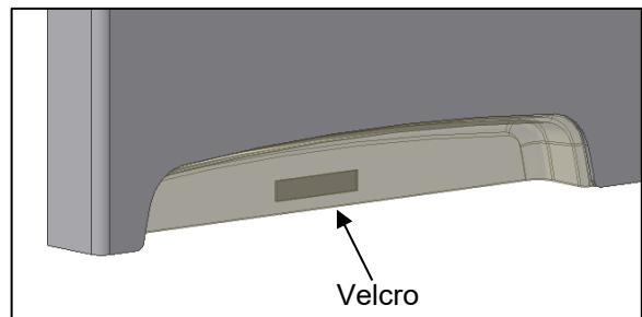
There is a small piece of velcro attached to backside of inside cover. After mounting of screws, move washbasin into bottom position. Remove protection paper from velcro, hold inside cover up and position close to outer cover and push against the wall until velcro sticks to wall.
