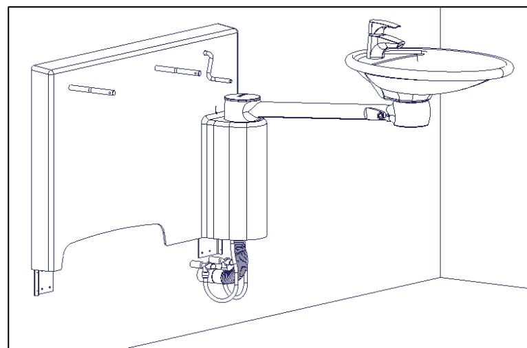
Connect drain pipe & connecting hoses.
