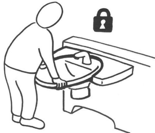
Ropox Swing Washbasin has a turning function, which means that it is **NOT** allowed to be used as a walking or standing support.
