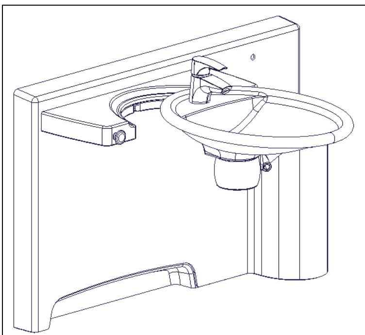
Test that washbasin freely can be swung into Dock-in and locks like it should. If washbasin is not positioned satisfactorily, fittings of Dock-in have to be loosened & either raised or lowered a little.
