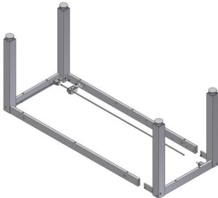
6.1.3 Now mount the two front fascias. Tighten the bolts securely.
