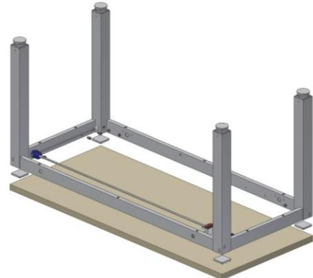
6.1.4 Place the frame on the table top and push the cover plates between legs and table top. Centre the frame in relation to the table top.
