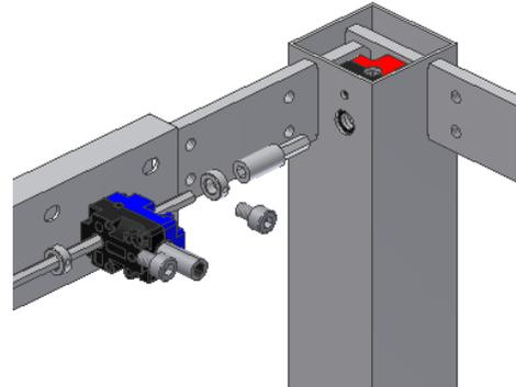
6.1.2 At the opposite end of the handle fit a stop ring on either side of the angular gear. Do not tighten the stop rings till the frame has been assembled.
