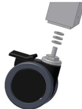
6.2.1 Mount the wheels. Do not forget to fit three washers on each wheel.
