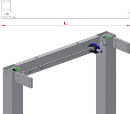
6.1.1 Check that the height (L) of all four legs is identical. May be adjusted on the hexagonal shaft. Place side fascias on a plane surface and mount legs. See label on legs.
