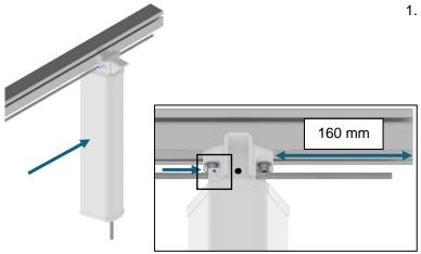
Slide on the first leg into the aluminum profile, and pass the hexagonal axle through the hole in the leg.
