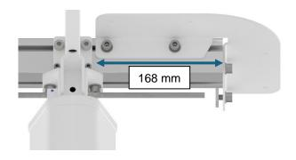
6. Slide the corner bracket into the aluminum profile. Tighten the screws **loosely**.
