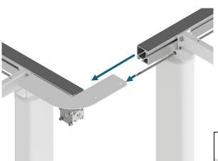
13. Assemble the two frames together in the corner bracket. The hexagonal axles must be placed in the gear from both sides. The ends must be flush.
