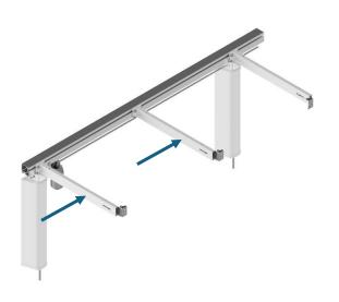
5. Place the next support arm brackets in the aluminum profile. The outermost bracket must be placed over the leg. Tighten the screws **loosely**.
