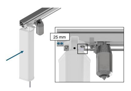
4. Slide the next leg into the aluminum profile, and pass the hex axle through the hole. Remember to mount the stop ring first. Tighten the screws **loosely**.
