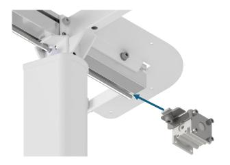
Slide the nut of the angular gear casing into the aluminum profile.
