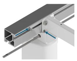
14. The support arm brackets can be leveled up and down with the set screws and supplied angle brackets, if needed.
