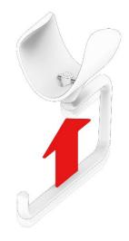
2. Once the cross-pin is free of the plastic, the holder can be rotated 90° and pulled back into the plastic bracket
