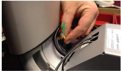
Connect the safety strip (the picture show Vision type E with 2 safety strips)
