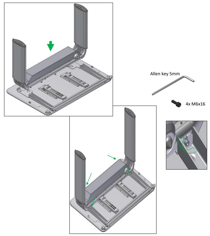
2. Mounting of tilting fitting of tabletop (not table A)
