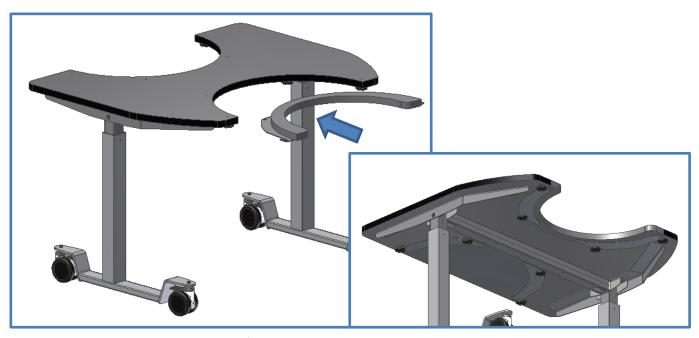
Push boomerang into cut-out section of tabletop. Tighten all 4 thumb screws which are in the tabletop.
