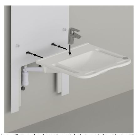
Mount the washbasin with the enclosed mounting parts for bolt mounted washbasins. Likewise, mount the mixer tap, but wait until later with mounting the hoses.
