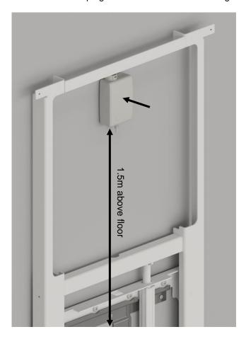
Remove the protective foil on the tape and fasten the power supply above the unit. Place it 1.5 m above the floor measured to the underside. Place it in the middle of the lifting unit.
