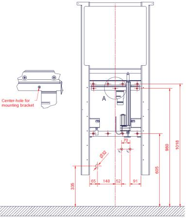
Place the unit in accordance with the water connection and drain as shown on the drawing.
