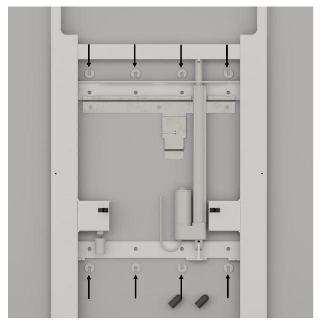
Push 8 spacers in behind the frame so that it has the right distance to the wall. Mark the 8 holes for fastening. Take the lifting unit down again and drill the holes in the wall.
