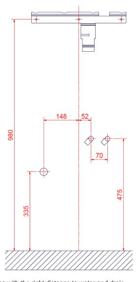
Fix the mounting bracket as illustrated on the drawing with the right distance to water and drain. Make sure that the mounting bracket is level.
