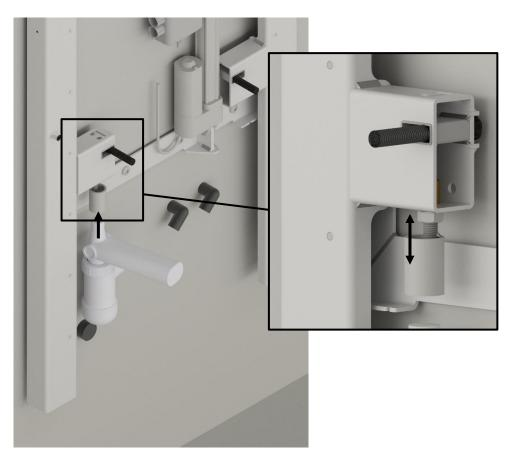
Install the siphon. Adjust the holder bracket according to the washbasin to be mounted. The height of the bracket depends on the height of the washbasin.
