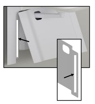
Cut the Velcro strips into two pieces, then remove the protective paper from the back. One side of the Velcro attaches to the metal frame, the other to the outer cover. Mount the outer cover as shown.
