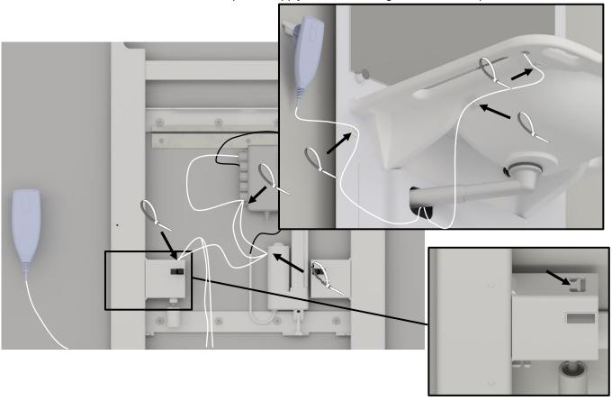
For the fixed control, it's recommended to lead the cables and fix them as shown, after the covers and washbasin has been mounted. The control cables are fixed to the mounted cable holders.
