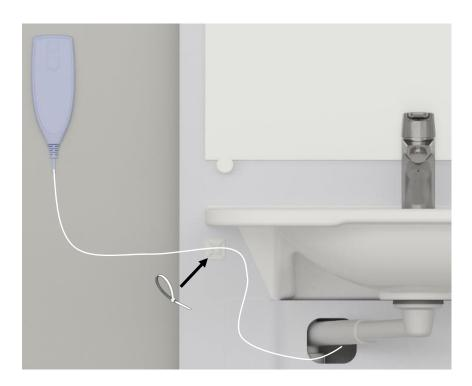
It's recommended to lead the cable and fix it as shown, after the covers and washbasin has been mounted. The control cable is fixed to the mounted cable holder. Ensure the cable can reach at least 1 meter from the last cable holder when extended.
