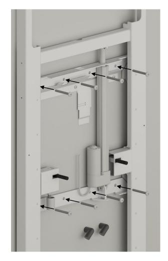
Use suitable rawlplugs and screws for the mounting.
