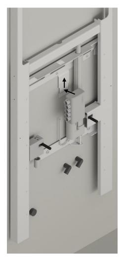
Mount the control box on the mounting bracket. Make sure that the small aluminum leg interlocks and locks the box in a fixed position.
