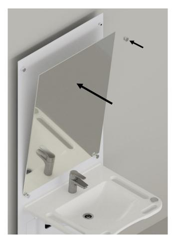
Remove the protective foil on the double-coated tape on the back of the mirror and fix it as illustrated. Press it firmly and make sure that the mirror is properly fastened so that the final mirror bracket can be mounted.
