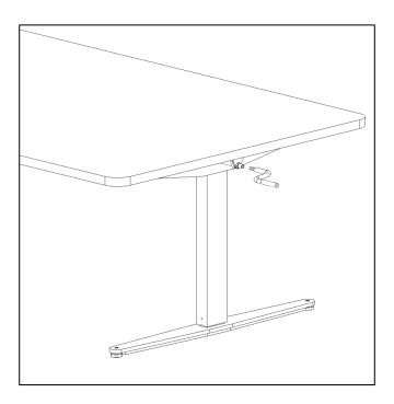
The height is adjusted by turning the hand crank on the side of the table manually. When turning the hand crank clockwise, the table will move upward.
