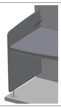
2. Mark holes on wall and floor through the three mounting fittings.
