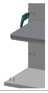
3. Drill holes in wall and floor.
