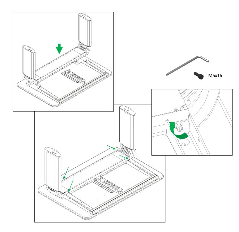
Mounting of tilting fitting of tabletop (not table A)
