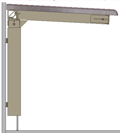
6.6.1 After placing the worktop on the frame you may have to compensate for the weight of the worktop if the frame is no longer horizontal from the wall to the front fascia.
