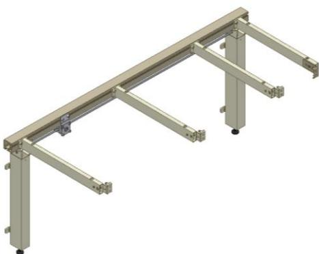
6.3.1 Place the frame against the wall and align it. Adjust the two threaded bolts under the legs to ensure that the frame is horizontal.
