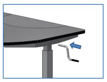
The height is adjusted by turning the handle on the side of the table manually. When turning handle clockwise, on the right side of the table, the table will move upward.
