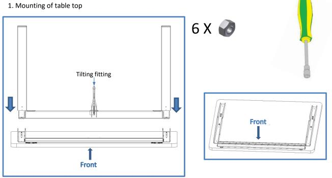
The tilting fitting on leg section must point towards the front of the table top
