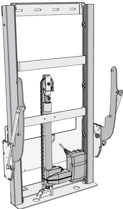
Place the lifting unit in the desired location. Be especially aware of the position of the drain, electrical and water inlet on the wall, as described previously.
