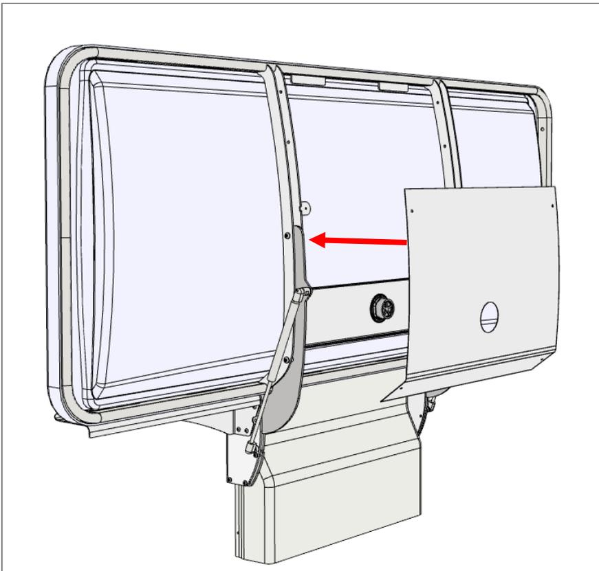
Place the cover plate between the two support arms underneath the Shower tray.
