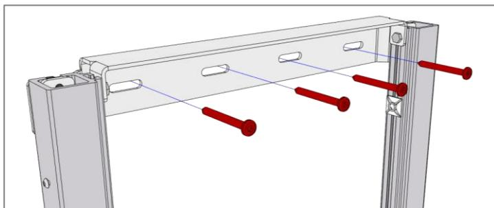
**Maximum pull force for each of the four screws in top of the unit: 45 kg**
