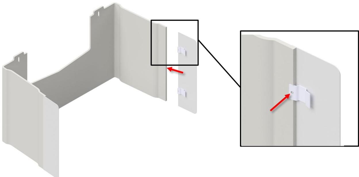
**b.** Lay down the outer cover, then mount the top
