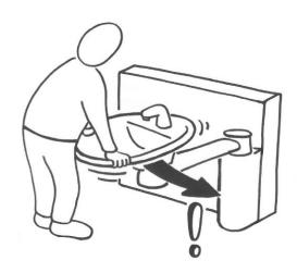
Ropox Swing Washbasin has a turning function, which means that it is **NOT** allowed to be used as a walking or standing support.
