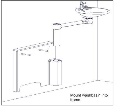
Move washbasin into top position. Mount 2 M5x6 screws under the cover each side. This is to avoid washbasin being pulled out.
