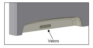
There is a small piece of velcro attached to backside of inside cover. After mounting of screws, move washbasin into bottom position. Remove protection paper from velcro, hold inside cover up and position close to outer cover and push against the wall until velcro sticks to wall.
