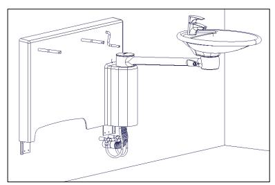
Connect drain pipe & connecting hoses.
