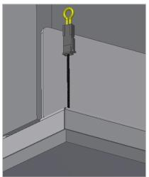
Place plug with yellow  $2,2k\Omega$  resistor on the right side of safety stop plate (shown from the front)
