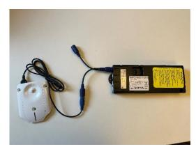
6.7.2 Insert the split-cable in the plug "**HS**" in the control box. Then, insert the adapter in one end of the split cable, and the button that came with the product, in the other
