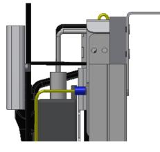
Attach cupboards to sliding frame and fasten
