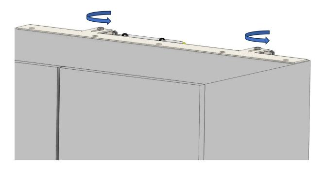
2. Adjust the leveling screws from behind the unit
