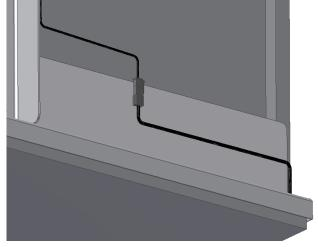
Connect the two cables for safety stop plates in the middle
