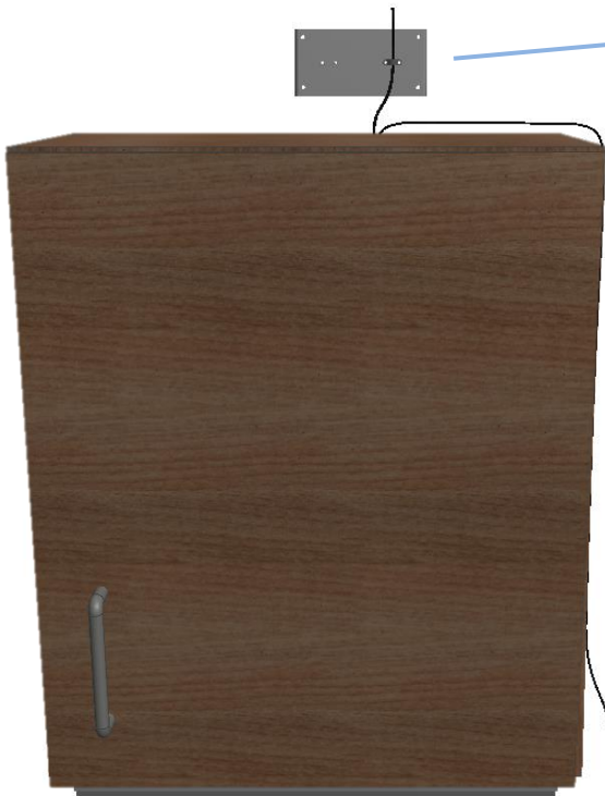
Mount cable relief for mains cable on wall
