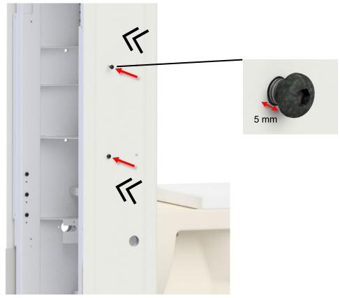
**C.** Slide the assembly onto the two screw heads and attach the assembly with the two M6x30 as shown.
