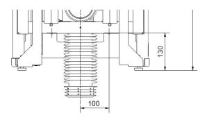
**b.** Connect water hose on wall outlet and electric outlet before securing frame to the wall
