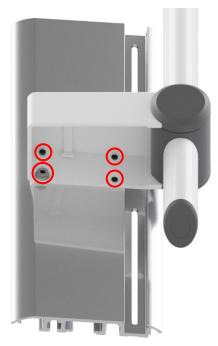
**b.** Make sure that the plastic cover is pressed as far onto the frame as possible. Mount 2x M6 buttonhead screws in the back holes on both sides. Leave 5mm of clearance between underside of screw head to the plastic cover.
