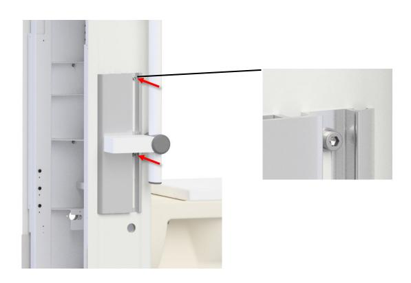
**d.** Test the toilet support arms in the horizontal direction. If they can twist significantly, dismount the assembly and leave <5mm between the underside of the screw head to the plastic cover. There should be no clearance between the aluminum bracket and plastic cover. Adjust until the support arms are properly fastened.
