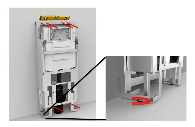
**a.** Line up frame with adjustment screws. Mark out 6 holes and drill holes for appropriate rawlplugs. Ensure that the center of the bottom 2 holes is at least 130mm above the floor
