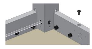
6.1.5 Fix the table top with screws through the holes of the fascias.
