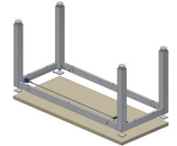
6.1.4 Place the frame on the table top and push the cover plates between legs and table top. Centre the frame in relation to the table top.
