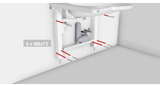
NOTE: Depending wall type, choose other suitable screws, as required. Max. load on upper screws: 71 kg / 156 lb /screw
