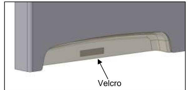
There is a small piece of velcro attached to backside of inside cover. After mounting of screws, move washbasin into bottom position. Remove protection paper from velcro, hold inside cover up and position close to outer cover and push against the wall until velcro sticks to wall.
