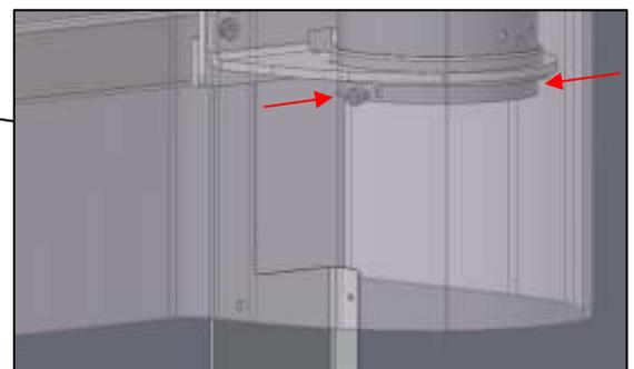
Connect drain pipe & connecting hoses.
