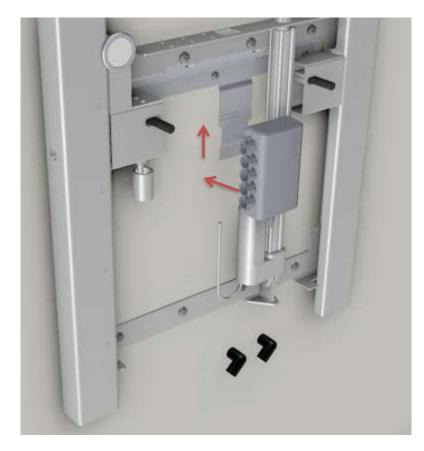
Mount the control box on the mounting bracket. Make sure that the small aluminium leg interlocks and locks the box in a fixed position.
