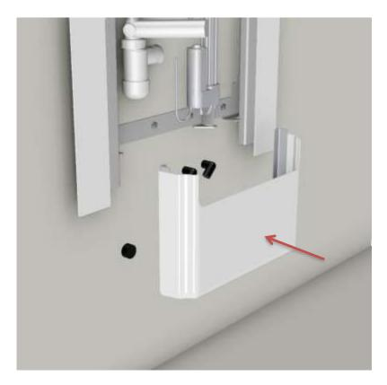
Remove the protective foil from the double-coated tape on the back of the brackets for the installation cover.
