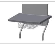
If the support legs have been purchased, they must be mounted before the lifting unit is mounted on the wall. See separate manual!
