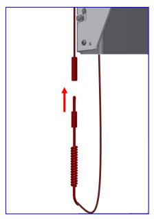
5. The water and drain can now be mounted. Drain hoses and water hoses come with the version with a sink.
