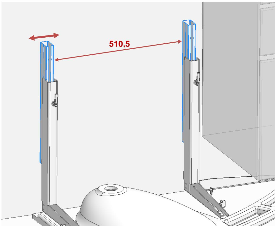
Fine adjustment of wall fitting – use legs on washbasin as a guide
