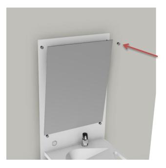
Remove the protective foil on the double-coated tape on the back of the mirror and fix it as illustrated. Press it firmly and make sure that the mirror is properly fastened so that the final mirror bracket can be mounted.
