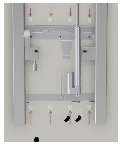
Push 8 spacers in behind the frame so that it has the right distance to the wall. Mark the 8 holes for fastening. Take the lifting unit down again and drill the holes in the wall.
