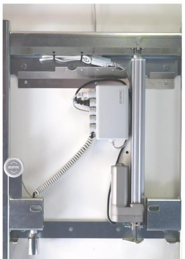
Connect the electrical system as illustrated. Fix the excess cable from the power supply on the mounting bracket with strips.
