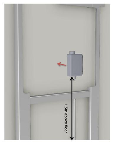
Remove the protective foil on the tape and fasten the power supply above the unit. Locate 1.5 m above the floor measured on the underside. Place it in the middle of the lifting unit.
