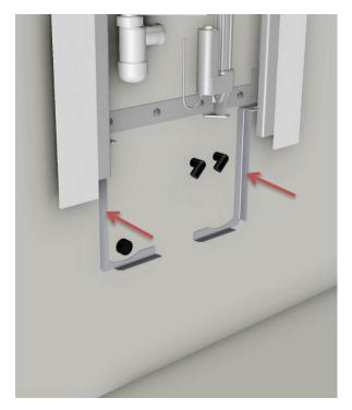
Remove the installation cover and push the brackets very firmly against the wall to make sure that the glue has good contact with the wall.
