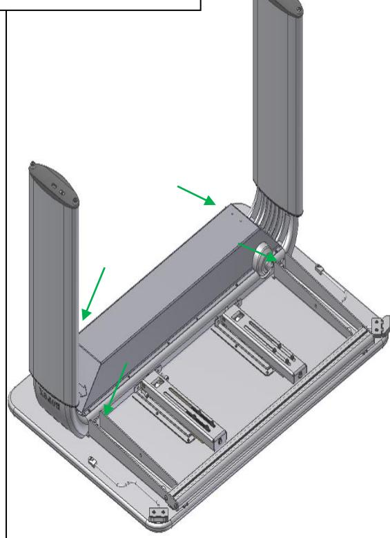
2. Mounting of tilting fitting of tabletop (not table A)
