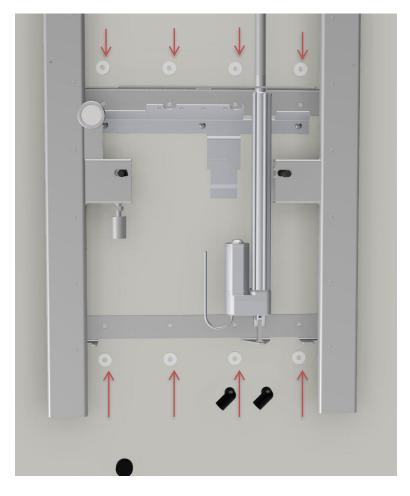
Push 8 (eight) spacers in behind the frame so that it has the right distance to the wall. Mark the 8 holes for fastening. Take the lifting unit down again and drill the holes in the wall.
