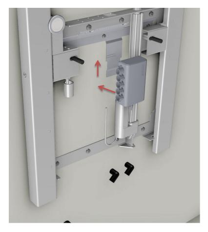
Mount the control box on the mounting bracket. Make sure that the small aluminium leg interlocks and locks the box in a fixed position.
