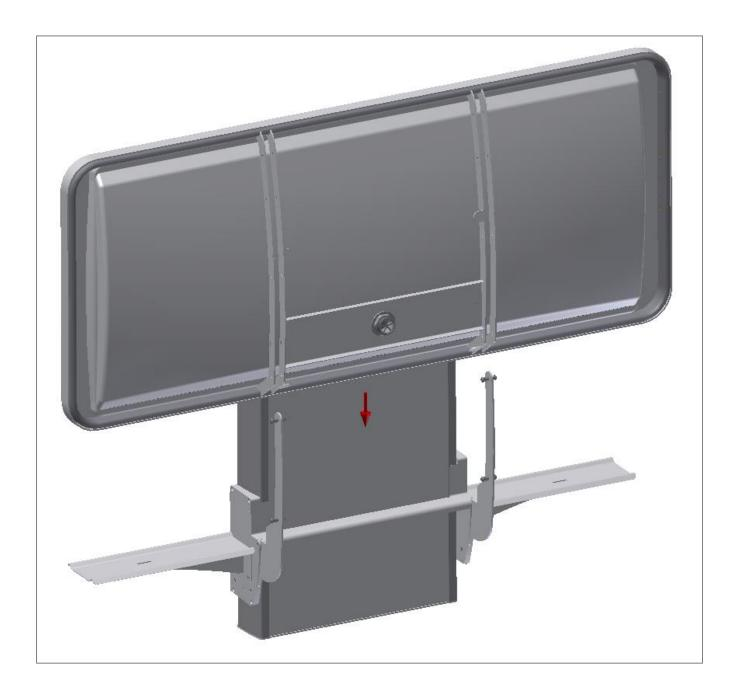
Fasten the Shower tray to the Lifting unit with 8 pcs. M8x12 through the bushings in the support arms.
