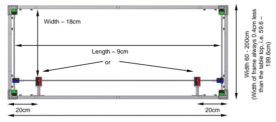
For table top length 60 - 300cm (Length of frame always 0.4 cm less than the table top, i.e. 59.6-299.6cm)
