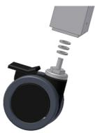
6.2.1 Mount the wheels. Do not forget to fit three washers on each wheel.
