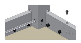
6.1.5 Fix the table top with screws through the holes of the fascias.
