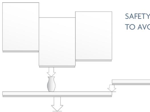
SAFETY STOP INSTALLED TO AVOID TRAPPING
