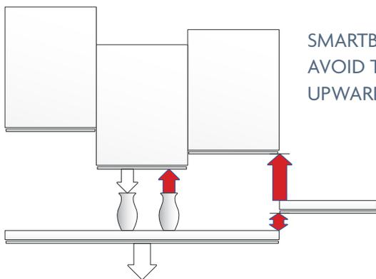
SMARTBOX INSTALLED TO AVOID TRAPPING DURING UPWARDS MOVEMENT \*
