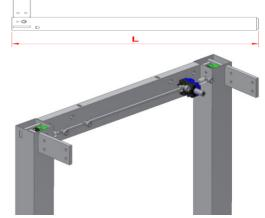
6.1.1 Check that the height (L) of all four legs is identical. May be adjusted on hexagonal shaft by means of the open-end wrench provided. Place side fascias on a plane surface and mount legs. See label on legs.
