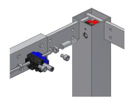
6.1.2 At the opposite end of the handle fit a stop ring on either side of the angular gear. Do not tighten the stop rings till the frame has been assembled.
